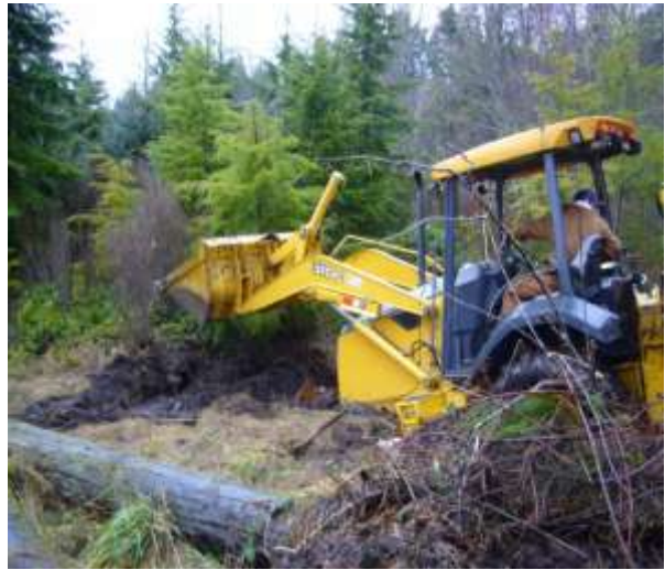
Figure3.1: Areas thought to be upland, turned out to be pockets of wood waste saturated with ground water and unsuitable for our exploration equipment access.
