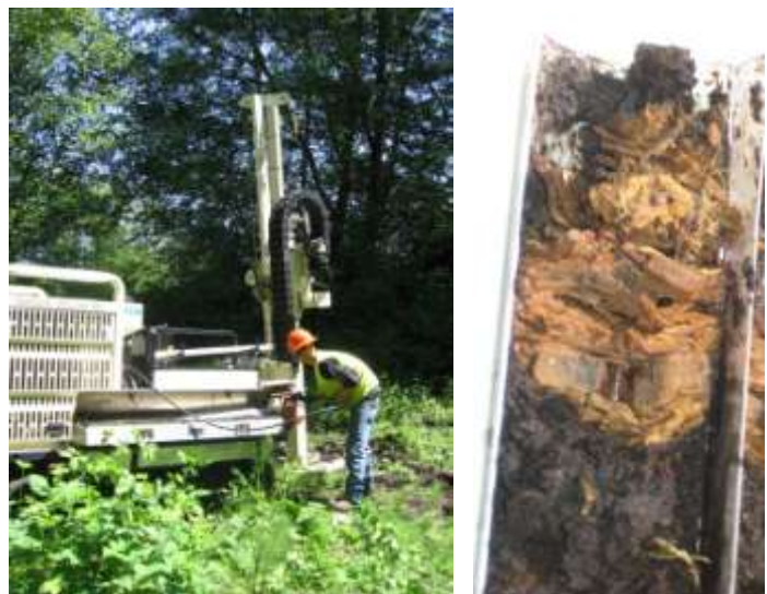
Figure 6.1: Left: Geoprobe used to take core samples of site; Right: Resulting core sample from project site with wood waste on top.
